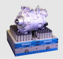
Perfect molding even with complex workpiece contours. These individual mold jaws are frozen by pneumatic actuators. Absolutely safe hold, even with low clamping forces.
